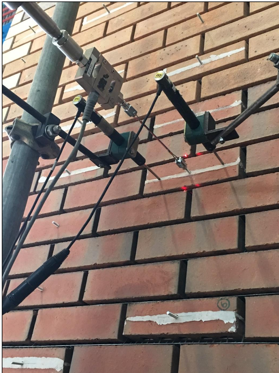
EXAMPLE OF PULL-OUT TEST SETUP
